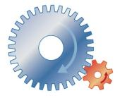
♦ If the first gear wheel is smaller (and has fewer teeth) than the second one, then the second (bigger) gear doesn't have to move as quickly to keep up with the smaller gear. So the second gear wheel turns more slowly than the first.
