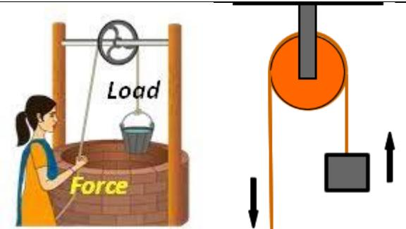
**Pulleys** have a rope or cable which goes over a wheel. This is pulled to lift, lower or move heavy objects.
